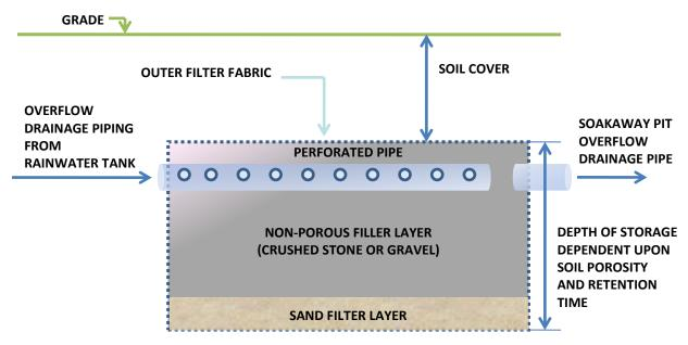
Figure D-2. Sketch of a typical soakaway pit (cross-section view)<sup>51</sup>
