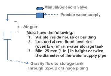
Figure 4-2. Schematic drawing of a top-up system with an air gap<sup>19</sup>
