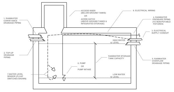
Figure 2-2. Rainwater storage tank schematic
