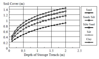
Figure D-3. Soil cover for soakaway pits, based on frost heave<sup>55</sup>
