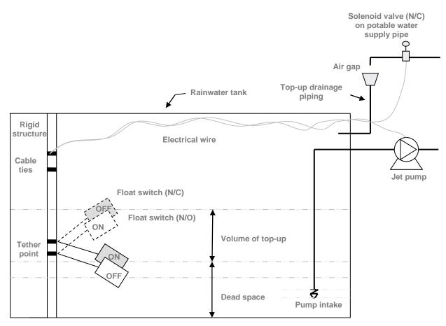
Figure 4-1. Components of an automatic top-up system
