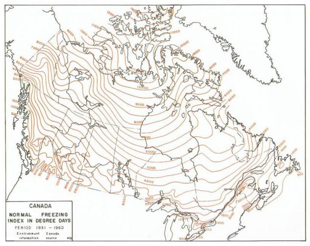
Figure A-3. Normal freezing index for Canada in degree days<sup>31</sup>
