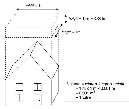
Figure 1-2. Theoretical volume of rainwater collected from a roof catchment
