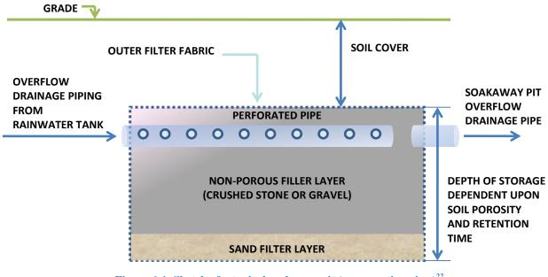
Figure 6-1. Sketch of a typical soakaway pit (cross-section view)<sup>22</sup>
