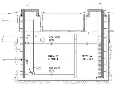
Figure 3-4. Rainwater storage tank with integrated settling and storage chambers<sup>13</sup>
