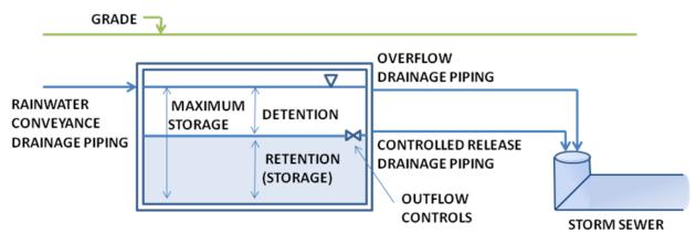
Figure D-1. Schematic of RWH system with outflow controls and controlled release drainage piping for stormwater management. ('DETENTION' is the volume of runoff to be slowly released to storm sewer. The remaining volume 'RETENTION' is used to supply rainwater to permitted fixtures)
