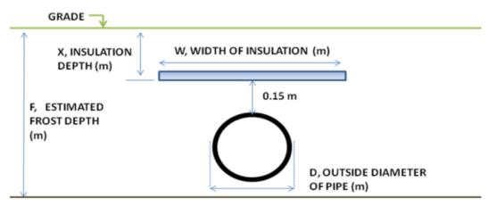
Figure A-5. Frost protection of pipe by horizontal insulation<sup>33</sup>
