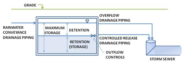
Figure 6-2. Schematic of RWH system with outflow controls and controlled release drainage piping for stormwater management. ('DETENTION' is the volume of runoff to be slowly released to storm sewer. The remaining volume 'RETENTION' is used to supply rainwater to permitted fixtures
