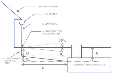
Figure A-4. Pipe conveyance (profile view)
