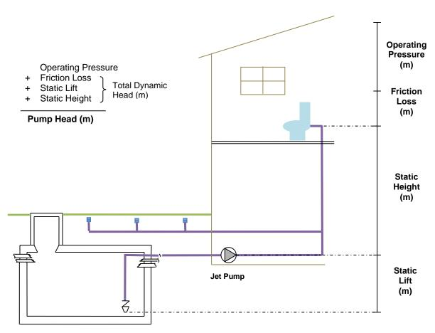
Figure 5-2. Components of Total Dynamic Head (TDH)
